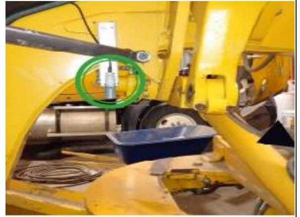
**Step 2:** Insert the orange 90-degree connector into the top of laser and tighten the waterproof ring until snug
